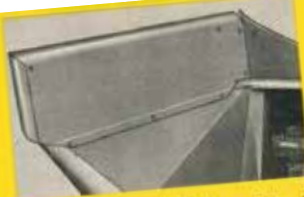
Flare sheet extension —Best when picking in extra tall corn or in varieties where ears break off easily; reduces ear loss over flare sheets.
