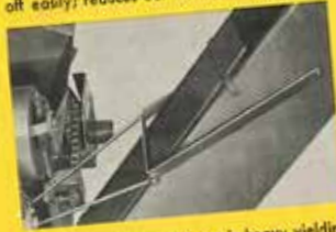
Wagon elevator cover —For use in heavy yielding corn where travel on rough ground may cause ears to bounce over the sides of the elevator.
